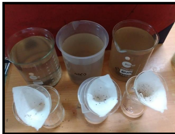
Figure 23: Flocculation-Coagulation with Seeds Powder and Filtration of the Sample
